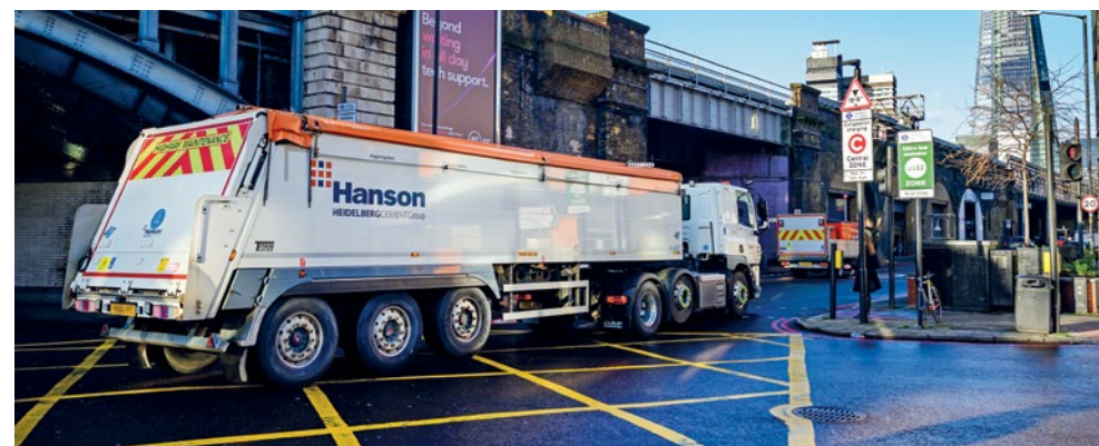
Walking floor articulated HGV delivering asphalt in London
