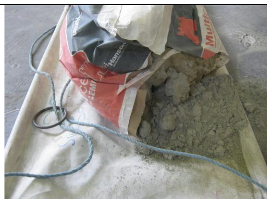
Specimen 1 – rupture to sidewall (2 nd drop in sequence)
