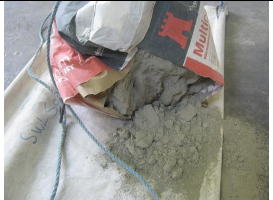
Specimen 3 – rupture to sidewall (2 nd drop in sequence)
