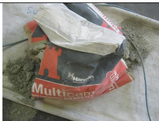
Specimen 2 – rupture to sidewall (2 nd drop in sequence)
